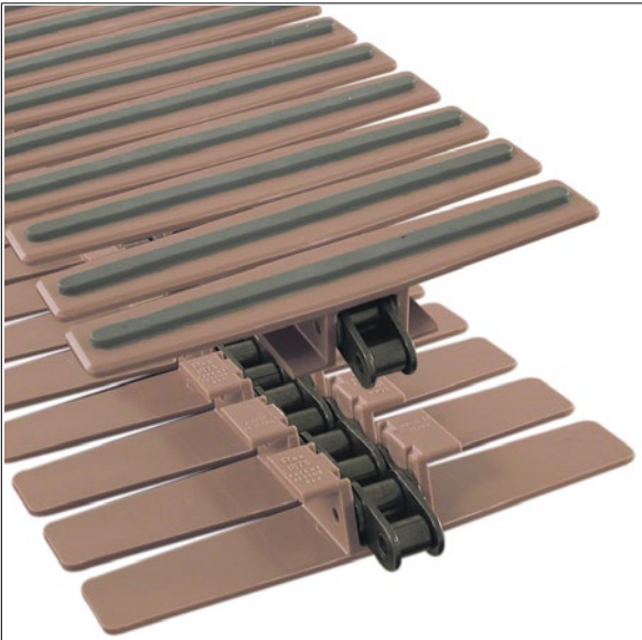
Photo shows 1873 TAB RubberTop TableTop Chain with High Friction Inserts and top plates molded in Low Friction (LF) material on Stainless Steel (SS) base chain.
